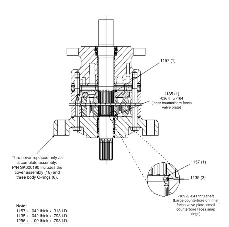
Fig. 3 Thru Shaft Option Snap Ring Replacement
