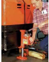
The J Series Toe Jack is an extremely rugged jack used here for lift truck service.
