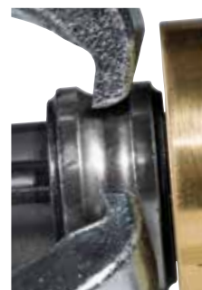
Lock on ball grooves and bearing races.
