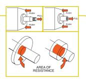
A shaft with a threaded end can be removed without damage by using one of our slide hammer, manual or hydraulic Bi-Directional™ Puller, in conjunction with the proper threaded adapter. Removal is easy! If the shaft to be removed has external threads, simply choose one of our female threaded adapters of proper size/thread. If the shaft has internal threads, simply choose the correct size male threaded adapter.
