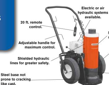
Modular design allows for quick interchange of pump with other modules.
