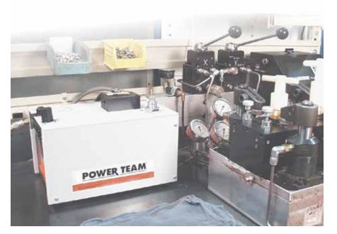
The PA60 used in a workholding environment.
