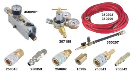
**No. 307159** – Pressure reducing valve. Allows use of bottled gases to operate jacks (works on CGA-580 Nitrogen/Argon/Helium bottles). Contains standard bottle fitting on inlet and <sup>1</sup>/<sub>4</sub>" industrial interchange (female) outlet. Wt., 4 lbs.
