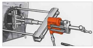
Combination of 50 ton capacity Bi-Directional Pullerand cup pulling attachment simplifies the removal of a final drive axle seal.
