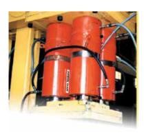
Four special order 500 ton, 24" stroke cylinders used in a swaging press for crimping 31/2" wire rope.
