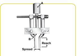
**↑ CAUTION** − These attachments may not withstand the full tonnage of the pullers they are used with. The shape and condition of the part being pulled affects the tonnage at which the jaws may slip off. Always select the largest attachment which will fit behind the part being pulled.
