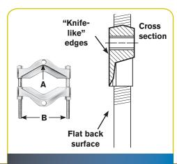
Attachment clamps down into V-groove to distribute load.
