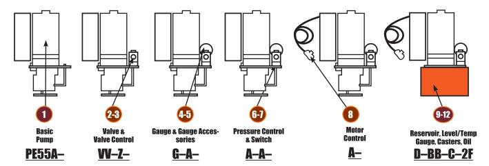
**Pump No. PE55A-VV-Z-G-A-A-A-D-BB-C-2F** is a 10,000 psi two-speed pump with a 115 volt, 50-60Hz, single phase, 14 hp, 12,000 rpm motor; a 9512 4-way solenoid valve with a 202778 remote hand control, a 9041 pressure gauge, no gauge accessories, standard pressure control, standard On-Off-Pulse motor control, 400630R9 2-gallon reservoir, a 350431 oil level/temperature gauge, 10494 casters, and 2 gallons of standard hydraulic oil.
