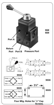
4-way 3-position (closed center) and (tandem center) manual valves with Posi-Check®
