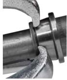
Tapered roller bearing on shaft.
