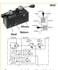
Pump mounted, 6-position detented 5-way manual dual valve. Rated pressure to valve "A" is 10,000 psi and valve "B" is 6,000 psi. Case pressure is 500 psi max.
