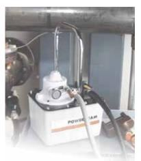
The PA17 used with a flange spreader
