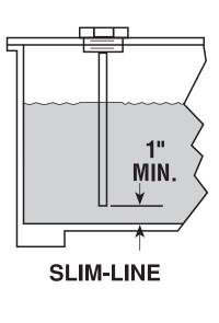
TYPICAL INSTALLATION Steel Support Rods are 12L14 Stainless Support Rods are 303CD
