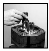
8) Remove the connecting shaft. Remove the thrust plate. Examine and replace if necessary. (See page 10). Remove the driven gear and the integral gear and drive shaft. Keep these together as they are a matched set. Examine and replace if necessary. (\*See page 10). Be careful not to damage the machined surfaces of the gears.
