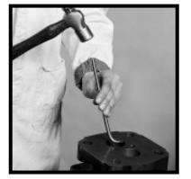
13) Grip the shaft end cover in a vise with the mounting face down. Remove double lip seal by inserting the special seal removal tool (see Tool List) into the notch between the double lip seal and the shaft end cover. Tap the seal out and discard. Remove and discard all
