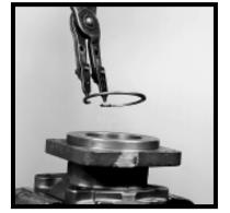
11) If the pump is equipped with an outboard bearing, place the shaft end cover in the vise with the mounting face up. Remove the snap ring with snap ring pliers. If a unit is equipped with a spiral-lock retaining ring, remove with a small screwdriver or awl.
