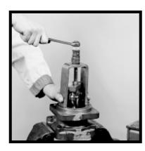
12) Use a bearing puller to remove the outboard bearing.
