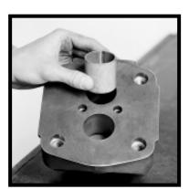
3) Grip shaft end cover in vise with mounting face down. Examine plug or plugs\* to be sure they're tightly in place.
