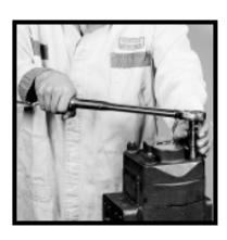
22) Thread the fasteners into the shaft end cover and tighten alternately or cross corner. Rotate the drive shaft with a 6" wrench to check for binding. If there is no internal binding, torque diagonally opposed fasteners to 200 ft. lbs. (2400 in. lbs.); 141 ft. lbs. (1700 in. lbs.) for PGP/ PGM315 models; 450 ft. lbs. (5400 in lbs.) for PGP/ PGM365.
