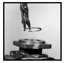
11) Install the snap ring in the groove to retain the outboard bearing.
