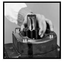
5) Carefully remove the drive and driven gears. Avoid tapping the gear teeth together or against other hardened surfaces. Keep these gears together because they are a matched set. Examine and replace if necessary. (See page 10). Remove the thrust plate from the bearing carrier. Examine and replace if necessary.
