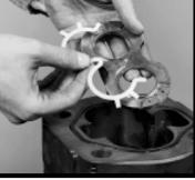
15) Slide the driven gear through the housing and into the bushing in the shaft end cover. Coat the steel sleeve tool with grease. Place the lightly-greased drive shaft inside the sleeve and slide both through the shaft end cover with a twisting motion, until the integral gear rests against the thrust plate. Avoid damaging the double lip seal. Remove the steel sleeve. Squirt clean oil over the gears.
