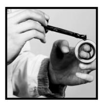
9) Before inserting a new lip seal in the shaft end cover, coat the outer edge of the lip seal and its recess with Permatex Aviation Form-A-Gasket<sup>™</sup> No. 3 non-hardening sealant or equivalent. With the metal side of the lip seal up, press it into the mounting flange side of the shaft end cover with an arbor press and bar (see Tool List on page 4). Be careful not to damage the lip of the seal. Press in until flush with the recess. Wipe off excess sealant.
