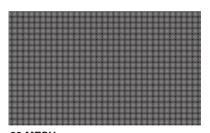
80 MESH Wire diameter .0055 Width of opening .0070 = 180 Microns
