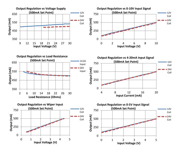
Note: All the above readings were taken with the DEC005000 adjusted for a .5 Amp maximum output at 100 Hz. A 14.6V supply was used for 12V coil tests and a 26V supply was used for 24V coil tests.
