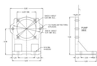
Machined to a 5.375 inch shaft centerline height
