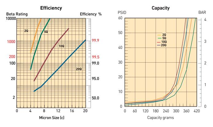
Results typical from Multi-pass tests run per test standard ISO 16889 @ 50 gpm to 60 psid terminal - 10 mg/L BUGL Refer to Appendix on pages 264-265 for relationship to test standard ISO 4572.
