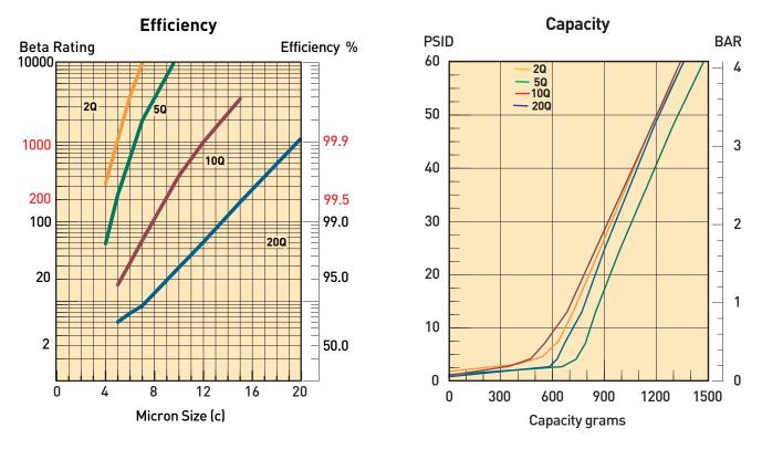
Results typical from Multi-pass tests run per test standard ISO 16889 @ 50 gpm to 60 psid terminal - 10 mg/L BUGL Refer to Appendix on pages 264-265 for relationship to test standard ISO 4572.
