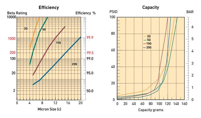
Results typical from Multi-pass tests run per test standard ISO 16889 @ 40 gpm to 60 psid terminal - 10 mg/L BUGL Refer to Appendix on pages 264-265 for relationship to test standard ISO 4572.
