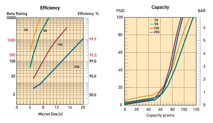
Results typical from Multi-pass tests run per test standard ISO 16889 @ 50 gpm to 100 psid terminal - 10 mg/L BUGL Refer to Appendix on pages 264-265 for relationship to test standard ISO 4572.
