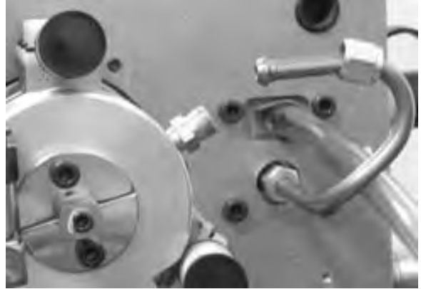
Figure 68. Motor Alignment to Pressure Tube
