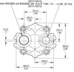
LEFT HAND ROTATION: PORT "A", TANK; PORT "B", PRESSURE RIGHT HAND ROTATION: PORT "A", PRESSURE; PORT "B", TANK
