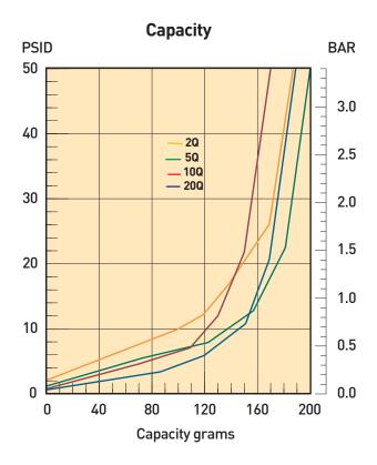
Results typical from Multi-pass tests run per test standard ISO 16889 @ 50 gpm to 50 psid terminal - 10 mg/L BUGL Refer to Appendix on pages 264-265 for relationship to test standard ISO 4572.
