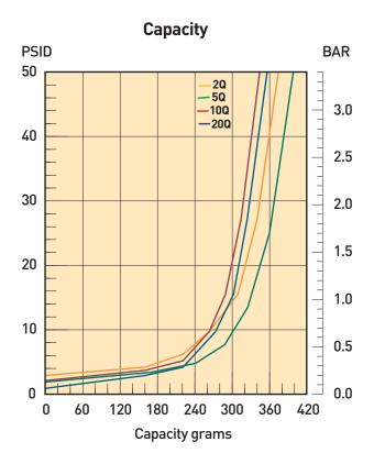
Results typical from Multi-pass tests run per test standard ISO 16889 @ 80 gpm to 50 psid terminal - 10 mg/L BUGL Refer to Appendix on pages 264-265 for relationship to test standard ISO 4572.
