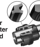
An extra-long inboard bearing surface insures lubrication from within the cylinder. Outboard of the bearing surface are two leakproof seals – The Lipseal and Wiperseal. The serrated Lipseal (primary seal) is completely self-compensating and self-relieving. It adjusts to mechanical deflections or any pressure variation from near-zero to rated operating pressure. The result is positive, no-leak sealing – regardless of conditions.
