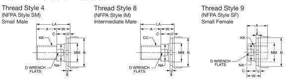
A high strength rod end stud is supplied on thread style 4 through 2" diameter rods. Larger sizes or special rod ends are cut threads. Style 4 rod ends are recommended where the workpiece is secured against the rod shoulder. When the workpiece is not shouldered, style 4 rod
