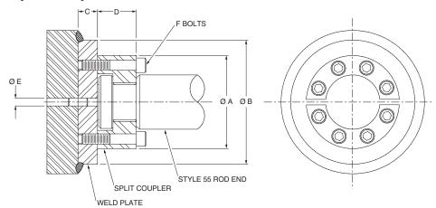
WARNING: Piston rod separation from the machine member can result in severe personal injury or even death to nearby personnel. The cylinder user must make sure the weld holding the weld plate to the machine is of sufficient quality and size to hold the intended load. The cylinder user must also make sure the bolts holding split coupler to the weld plate are of sufficient strength to hold the intended load and installed in such a way that they will not become loose during the machine's operation.
