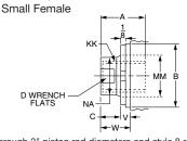
ends are recommended through 2" piston rod diameters and style 8 rod ends are recommended on larger diameters. Use style 9 for applications where female rod end threads are required. If rod end is not specified, style 4 will be supplied.
