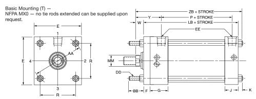
Style TB (NFPA MX3). Head Tie Rods Extended, illustrated: Style TC (NFPA MX2), Cap Tie Rods Extended; and Style TD (NFPA MX1), Both Ends Tie Rods Extended are also available. All "T" styles can be dimensioned from Style TB drawing at right.
