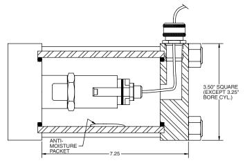
**Style D** — For LDT Basic and Intergral Cap. Specify connector type (not available on 2" bore).
