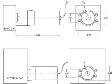
**Style F** — For LDT and LRT For 4" bore and larger only. Use Style A for  $2^{1}/_{2}$ " and  $3^{1}/_{4}$ " bore.
