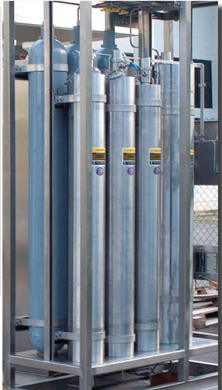
Typical application of Gas Bottles and linear transducer-equipped Piston accumulators in an oil well control assembly – Courtesy of Control Automation PTE LTD."
