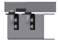
5. Place the (4) 13" x 2" x 1" rubber mounting pads on the base panel as shown in exploded view.
