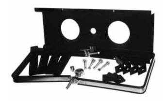
The ABK-340-C Mounting kit comes standard with the A3070 and the A4070 hydraulic upright tanks. Mounting kit includes: Mounting base panel, carbon steel strap assembly with springs and rubber mounting pads. Also supplied is the ASK-200 mounting kit which includes four pre-drilled powder coated mounting angles, plated bolts, washers, nyloc-nuts, four plated springs, and four mounting pads. Also includes filter/breather cap and auxillary vent. Ships in one carton.
