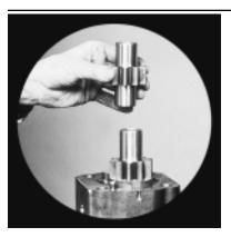
5) Carefully remove the drive and driven gears, without allowing the teeth to come into rough handling contact. Keep these gears together, because they are a matched set. Examine and replace if necessary. (See page 9.)
