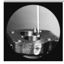
4) If plug or check valves are being replaced, screw in new parts tightly. Stake the plug with a prick punch at both ends of the screwdriver slot and around the edges. Screw the check valves in tightly with the tool. Peen edge of hole 1/32" to 1/16" with 1-1/2" diameter steel ball.
