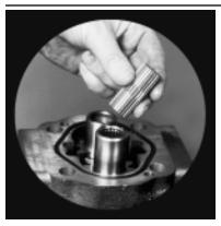
7) Remove the drive gear connecting shaft. For multiple assemblies only.
