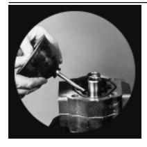
14) Slide the first section gear housing over the gears and tap it with a soft hammer until it rests tightly against the shaft end cover.
