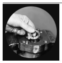
5) ASSEMBLY STEPS 5, 6, 7, 9 AND 11 APPLY TO THE SHAFT END COVER, BEARING CARRIERS, AND THE PORT END COVER. If the ring seals are being replaced, insert into the bottom of drive the gear bearing bore. The notch in the ring seal MUST BE VISIBLE. This is a check to be certain that the notched side is next to the bearing.
