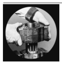
8) Lift or pry off the first section gear housing. Be careful not to damage machined surfaces. If the thrust plate remains in the gear housing, remove as described in Step 3.
