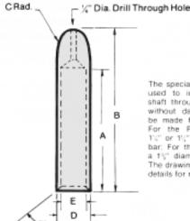
The special steel sleeve is used to insert the drive shaft through the lip seal without damage and can be made from bar stock: For the P30/P31, use a 1%" or 1%" diameter x 4%" bar; For the P50/P51, use a 1%" diameter x 5%" bar. The drawing and chart give details for making this tool.
