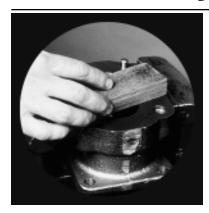
1) Stone off all machined surfaces with a mediumgrit, carborundum stone.
