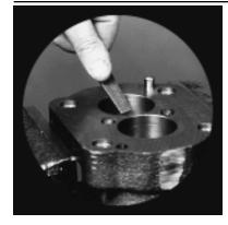
2) If the bearings have been removed, deburr bearing bores. Rinse parts in a solvent. Air blast all parts and wipe with a clean, lintless cloth before starting assembly.
