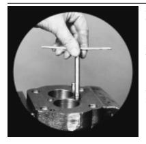
3) Grip the shaft end cover in a vise with the mounting face down. Examine the plug or the 2 check valves to be sure that they're tightly in place. Replacement is necessary only if parts are damaged. Remove with a screwdriver or a special check valve tool (see Tool List page 10).
