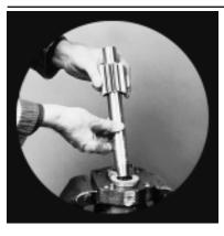
12) Insert the splined end of the drive shaft into the special steel sleeve (see Tool List page 10). Lightly grease the drive shaft and sleeve. Insert the integral gear and drive shaft with sleeve into the shaft end cover with a twisting motion. Be careful not to damage the double lip seal. Push down carefully until the gear rests against the thrust plate. Remove the steel sleeve. Insert the driven gear.
