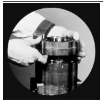
4) Lift the gear housing from the gears. Take care not to damage machined surfaces.
