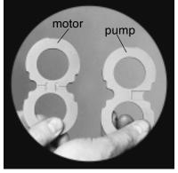
8) Check all thrust plates for wear. Replace if necessary (see page 9). Note that the thrust plates for pumps and motors are different. Pump thrust plates have a single relief pocket and must be installed with this groove on the high pressure side. Motor thrust plates are grooved on both sides.
