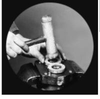
10) With the pocket seals facing down, place the thrust plate over the bearings in the shaft end cover. Tap thrust plate with a soft hammer to about 1/32" from the machined surface.
