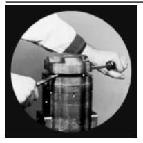
3) Lift off the port end cover. If necessary to pry loose, refer to caution note. If the thrust plate remains
