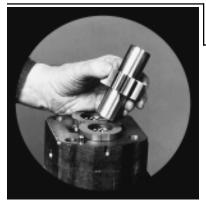
17) Insert the drive and the driven gears of the second section into their respective bearings.
