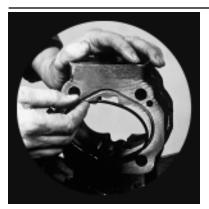
13) Grease the new gasket seals and insert them into the grooves in both sides of all gear housings. For the PGP031/051 - Examine all dowel pins. (See page 9.)\* Before inserting a pin, make certain that the hole is clean and free from burrs. Start the pin into the hole gently and straight, tapping lightly with a soft hammer.
