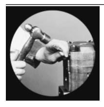
1) Mount the pump in a vise with the shaft end pointing down. Index mark all sections with a punch. Be sure to align these marks when reassembling.
