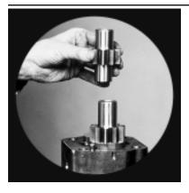
9) Remove the driven gear and the integral gear and drive shaft. Keep these together as they are a matched set. Examine and replace if necessary. Be careful not to damage the machined surfaces of the gears.
