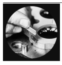
11) Cut 4 pocket seals approximately 1/4" long from the pocket seal strip. Insert one pocket seal into each of the slots in the thrust plate. Push each pocket seal all the way in so that it touches the roller bearings. Tap the thrust plate down firmly against the machined surface with a soft hammer. Use a sharp razor blade to trim the exposed end of the pocket seal square and flush with the thrust plate.
