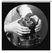
15) With the thrust plates mounted on the bearing carrier (as in steps 9, 10, 11), position it on the gear housing so that the roller bearings receive the journals of the drive and driven gears. Make sure that the drain port in the bearing carrier is on the suction or inlet side if the unit is being built as a pump. (Motors do not have drain vents in the bearing carrier.) Make sure that the index marks are properly aligned. Insert dowel pins (PGP031/051 only). For multiple assemblies only.
