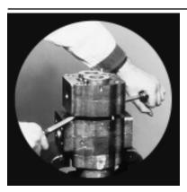
6) Lift or pry off the bearing carrier carefully to prevent damage to contact face and edges.
