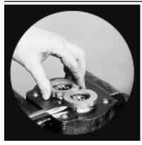
10) Pry the thrust plates from the shaft end cover, port end cover, or bearing carrier with a screwdriver or similar tool. Avoid distorting the thrust plates. Visually inspect thrust plates for wear or damage. Replace if necessary. (See page 9.) Remove and discard all rubber pocket seals and gasket seals.
