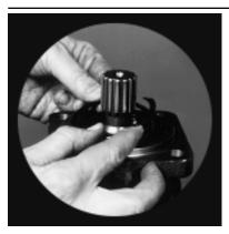
22) If the unit is equipped with an outboard bearing, guide the bearing into its recess in the shaft end cover. This is not a press fit. Insert the snap ring into its groove to retain the outboard bearing.
