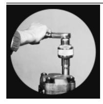
2) Remove the 4 cap screws on single units, or the 4 hex nuts, studs, and washers on multiple units with a socket wrench.
