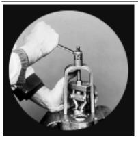
11) Examine all roller bearings for scoring, spalling, or pitting. If replacement is necessary, remove the bearings with a bearing puller.
