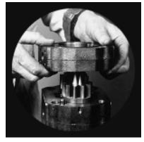
18) Slide the second section gear housing over the gears and tap it tight against the bearing carrier with a soft hammer. Be careful not to pinch the gasket seal. Squirt oil over the gears to provide initial lubrication when pump is started.
