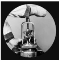
**14)** Use a bearing puller to remove the outboard bearing.
