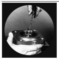
13) If the pump is equipped with an outboard bearing, place the shaft end cover in a vise with the mounting face up. Remove the bearing snapring with a small screwdriver or awl.
