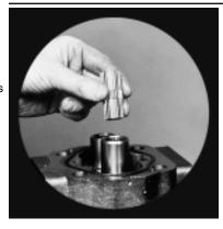
**16)** Insert the connecting shaft in the spline of the drive gear.
