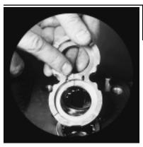
9) Grip the shaft end cover in a vise with the mounting face down. Cut 2 pocket seals 7/32" long from the pocket seal strip. Grease these pocket seals well and insert them into the middle slots on the reverse side of the thrust plate.
