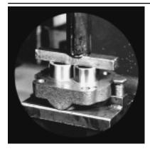
6) If any bearings have been removed from the shaft end cover, port end cover, or bearing carrier, replace the bearings by pressing them into the bearing bore with an arbor press.
