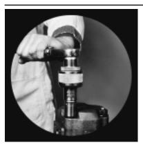
21) After the fasteners are tight and you are sure there is no internal binding, torque the diagonally opposite fasteners to 200 ft. lbs. (2400 in. lbs.).
