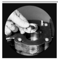
advisable to replace ring seals when rebuilding the unit. To replace, remove the drive gear bearing with a bearing puller, and remove the iring seal from the bottom of the bearing bore.
