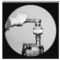
20) Thread the 4 fasteners (cap screws and washers, or studs, washers, and nuts) into the shaft end cover and tighten alternately or cross-corner. Rotate the drive shaft with a 6" wrench to make certain there is no binding in the pump.
