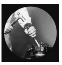
15) With the mounting face down, remove the double lip seal by inserting the special seal removal tool (see Tool List Pg. 10) into the notch between the double lip seal and the shaft end cover. Tap the seal out and discard.
