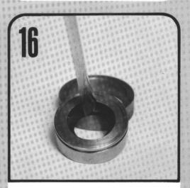
Tap the seal from the seal retainer and discard. Clean seal bore with solvent to remove old sealant. If bore is scored, smooth with fine grade emery paper. It is generally advisable to replace the seal retainer.
