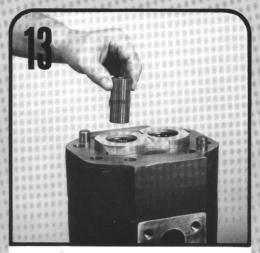
Insert the connecting shaft in the spline of the drive gear.
