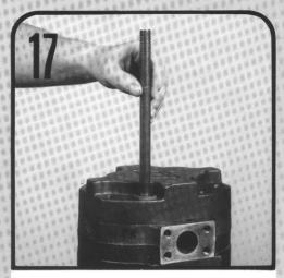
Thread the 8 fasteners (cap screws and washers, or studs and nuts) into the shaft end cover and snugup alternately or cross-corner. Rotate the drive shaft with a 6" wrench to make sure there is no binding in the pump.
