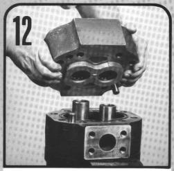
Position the bearing carrier with thrust plates on the gear housing so that the roller bearings receive the journals of the drive and driven gears. Make sure that the index marks (See Step 1, Disassembly) are properly aligned. Tap the bearing carrier tight with a soft hammer.
