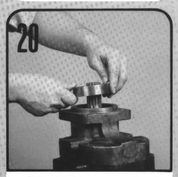
Drop in the spacer or outboard bearing. The outboard bearing may need to be lightly tapped into the bearing bore.
