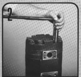
Remove the 8 cap screws or hex nuts and washers with a socket wrench.
