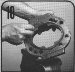
Grease the new gasket seals and insert them into the grooves in both sides of all gear housings.
