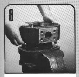
Lift or pry off the first section gear housing. Be careful not to damage machined surfaces. Remove thrust plate as described in step 3.
