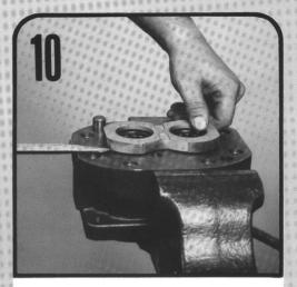
Pry the thrust plate from the shaft end cover, portend cover, or bearing carrier with a screw driver or similar tool. Avoid distorting the thrust plate. Remove and discard all rubber pocket seals and gasket seals.
