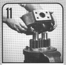
Slide the first section gear housing over the gears and tap it with a soft hammer until it rests tightly against the shaft end cover. Be careful not to pinch the gasket seal. Squirt oil over the gears to provide initial lubrication when pump is started.
