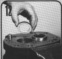
It is generally advisable to replace ring seals when rebuilding unit. To replace, remove the drive gear bearing with a bearing puller and remove ring seal from the bottom of bearing bore. Check all ring seal bores in unit for abnormal wear. If worn, replace those sections.
