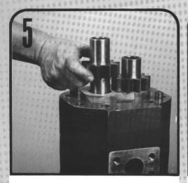
Remove the drive and driven gears. Keep the gears together because they are a matched set. Examine and replace if necessary. See below\*.
