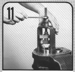
Examine all roller bearings for wear and discoloration. If replacement is necessary, pull the bearings with a bearing puller. Any sign of wear or discoloration calls for replacement. Remove bearings with a bearing puller.
