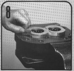
Cut 4 pocket seals approximately 7/16" long from the pocket seal strip. Insert one pocket seal into each of the slots in the thrust plate. Push each pocket seal all the way in so that they touch the roller bearings. Tap the thrust plate down firmly against the machined surface with a soft hammer. Use a sharp razor blade to trim exposed end of the pocket seal square and flush with the thrust plate.
