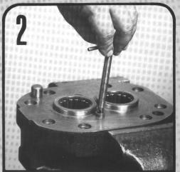
Grip the shaft end cover in the vise with the mounting face down. Examine the plug or 2 check valves, whichever is used, to be sure they are tightly in place. Replace only if parts are damaged or missing. Check valves can be removed with the special tool (see tool list). Screw in new valve with the tool until tight. Peen with a 1½" steel ball to secure.
