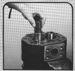
Remove the connecting shaft.
