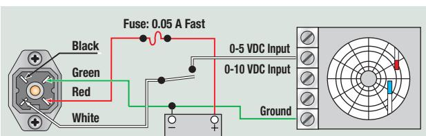
Schematic 4: 0-5 Vdc or 0-10 Vdc connection using target external power supply
