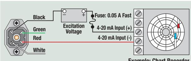
Schematic 3: 4-20 mA connection using target external power supply
