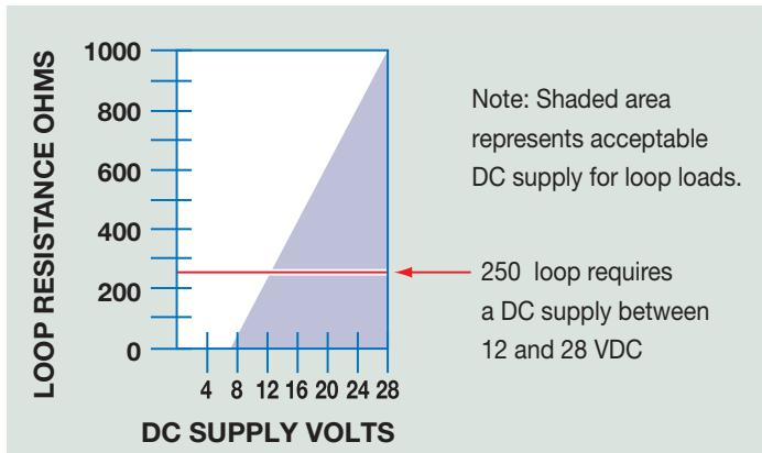
Figure 1. Load Limitations (4-20 mA Output Only)
