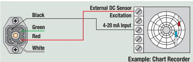
Schematic 1: 4-20 mA connection using target power supply
